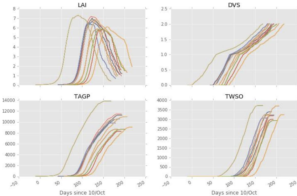
**Figure 3-11 Detailed analysis of the behavior of the simulation results for maturity group 5: results shown are leaf area index (LAI), development stage (DVS), total crop biomass (TAGP) and crop yield (TWSO) (biomass and yields expressed in 0% moisture), different colors represent different experiments**
