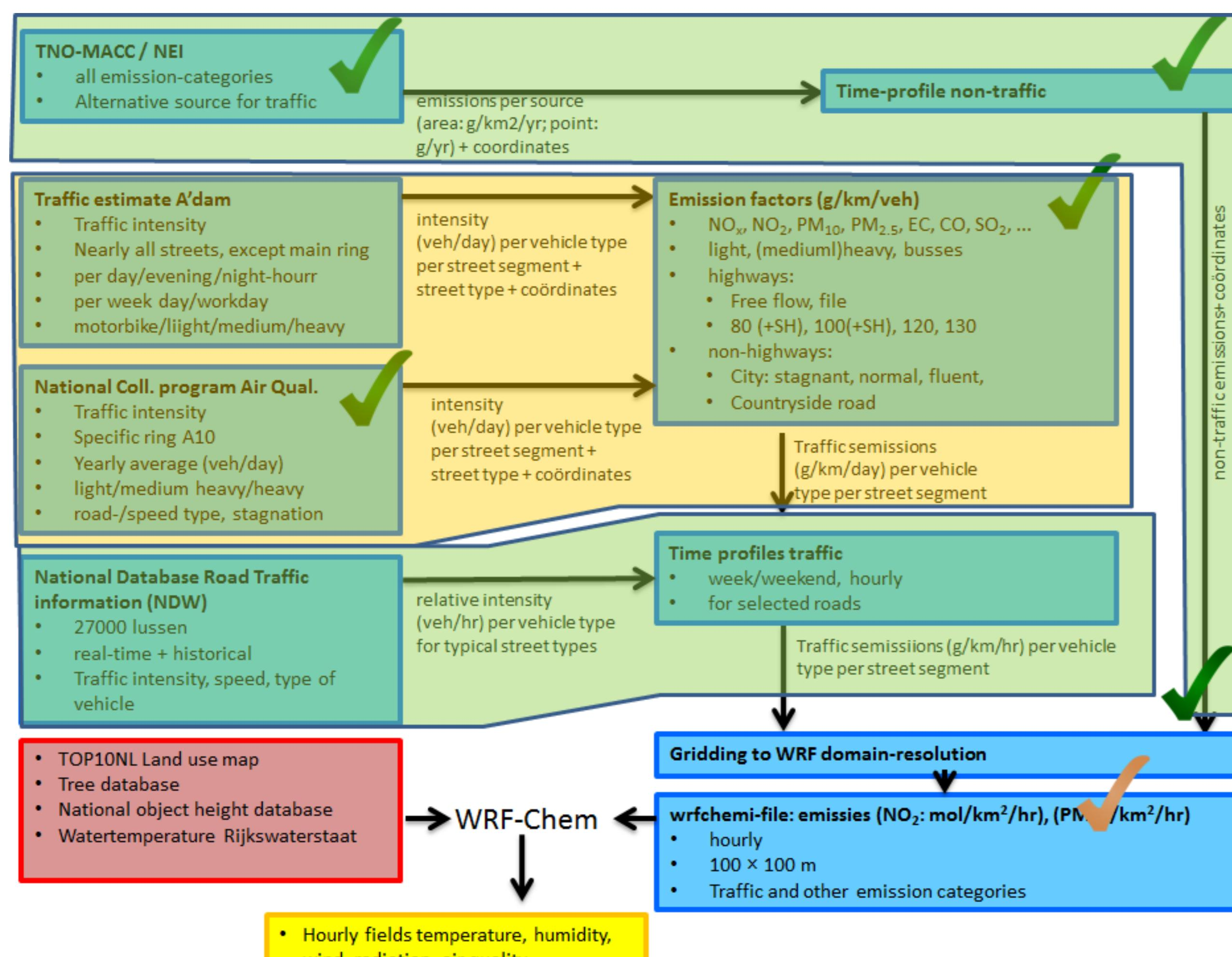
Figure 1. Organization of the NO<sub>x</sub> and heat emission fields into WRF-Chem
