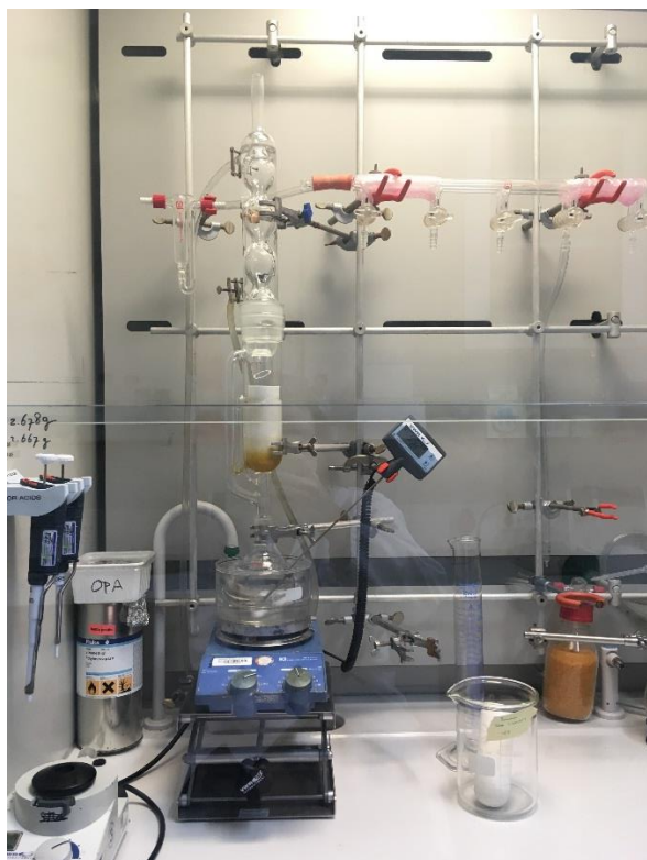
Figure 10: Soxhlet apparatus setup
