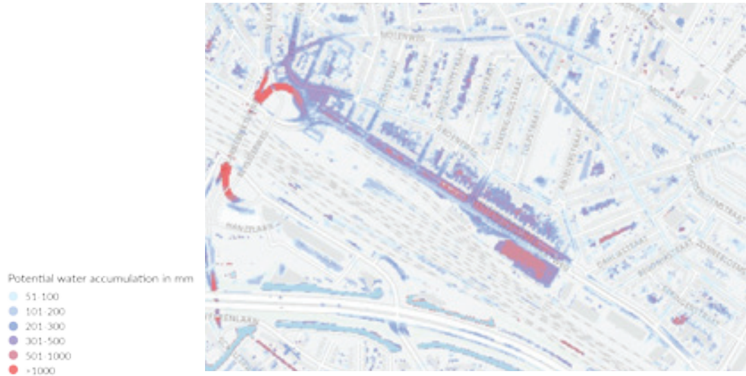
Figure 19. Water accumulation in Assendorp (Tauw, 2013)
