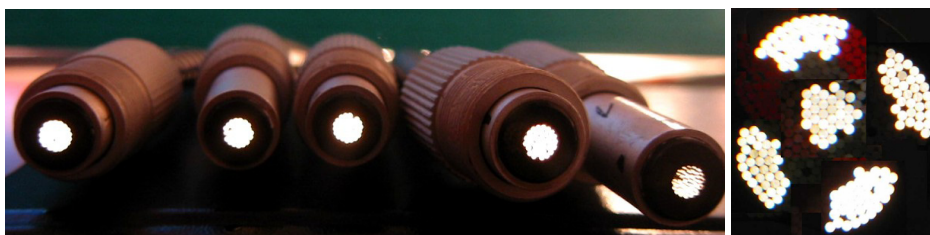
Figure 3.3.5. Branches of the 5-branch fiber (left) and its common end showing each illuminated section (right): middle is used for laser guiding.
