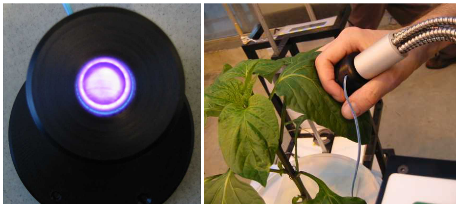
Figure 3.3.4. Performing a UV induced measurement (right) with the sample holding clip containing the UV illuminating head (left).
