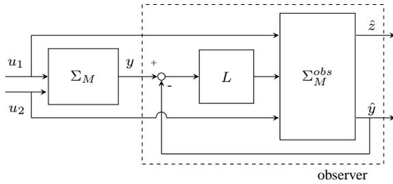
Fig. 1. Schematic overview process ( $\Sigma_M$ )–observer
