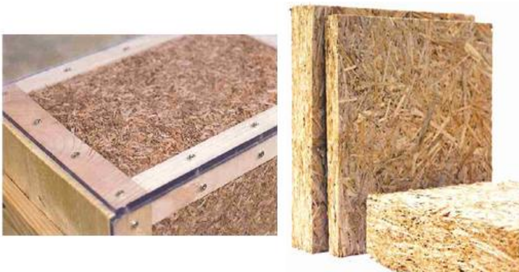
Figure 5. Blow-in insulation material from 100% cattail in a display case, and construction panels made of cattail (adapted from Wichtmann et al., 2016).
