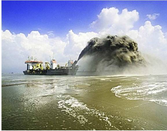
Figure 1.2: Trailing suction hopper dredger rainbowing
