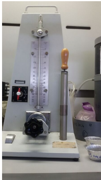
Figure 2.3: Pycnometer used for the porosity calculations. The air tight chamber is behind the black knob, the pump can be seen on the right and the switch on the left (red)
