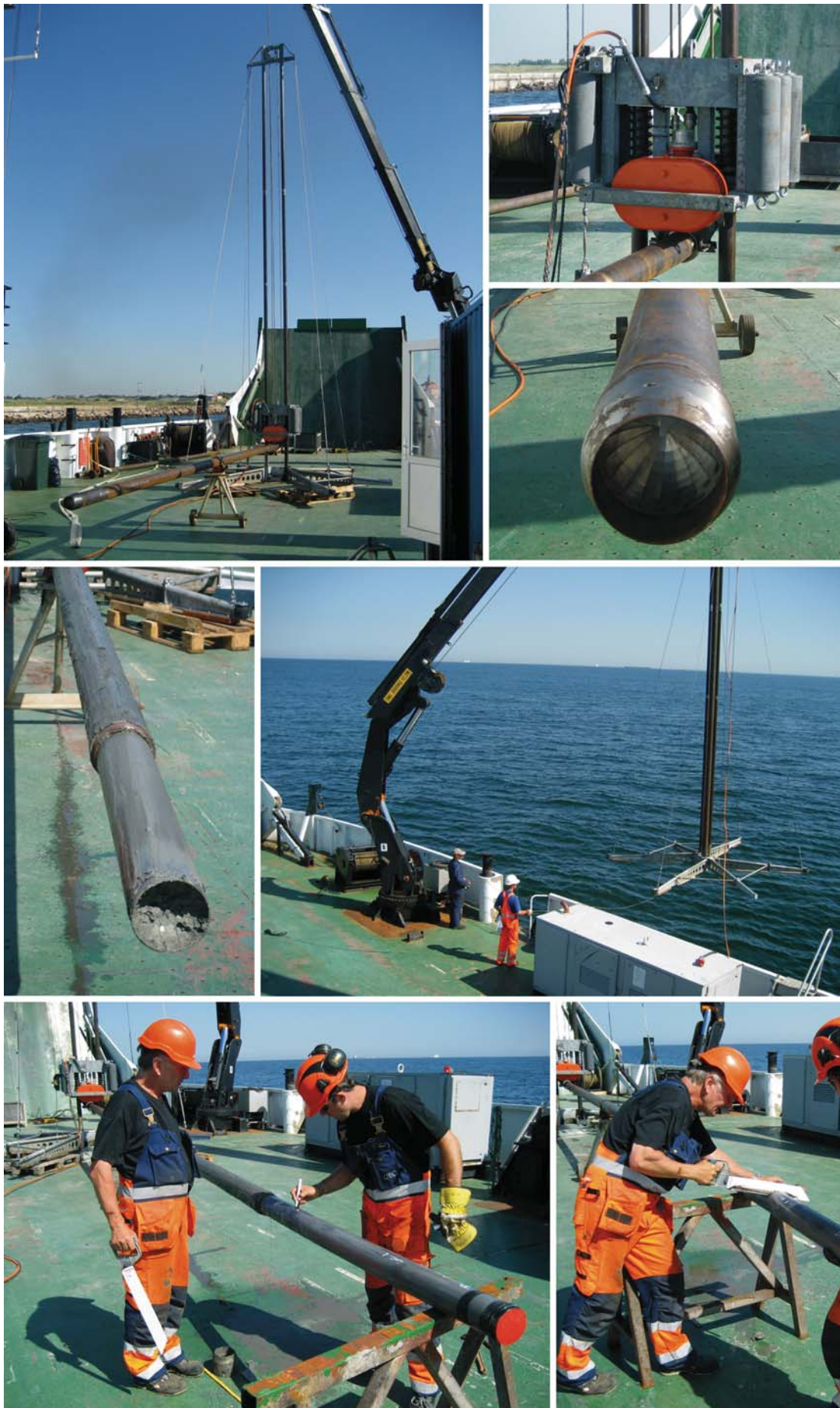
Figure 9.10: Retrieval of sediment cores in the Fehmarnbelt project for geological and palaeoenvironmental investigations (after Flemming et al. 2014, Fig. 4.10).
