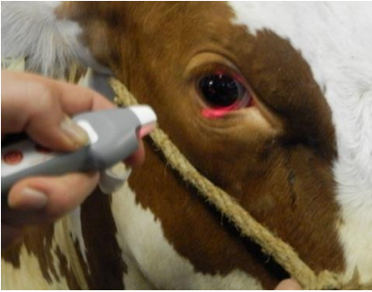
Figure 1: Non-contact body temperature measurement on the bovine eye with the Thermofocus Animal®
