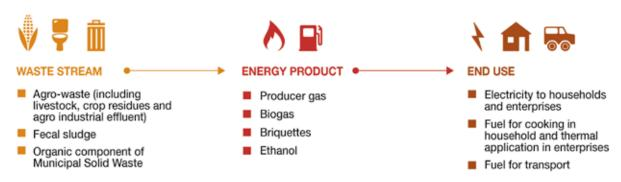
Figure 1. Waste-to-energy process framework (Otoo and Drechsel, 2017)
