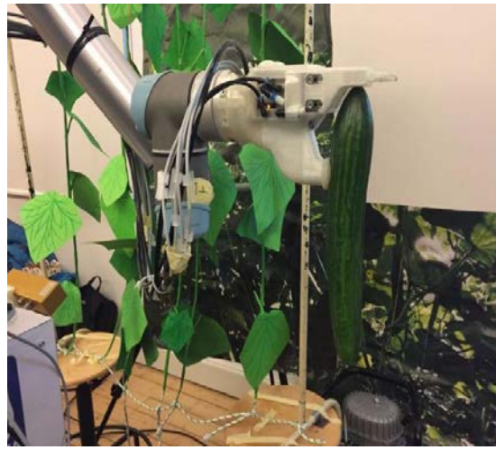
Figure 4.8 Cucumber harvesting robot for greenhouse application. Photo courtesy of the robot KasPR, Minor Robotics of the TU Delft
