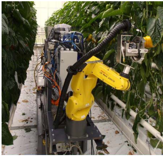
Figure 4.7 Sweep pepper harvesting robot in the greenhouse. Photo courtesy of EU-Sweeper project
