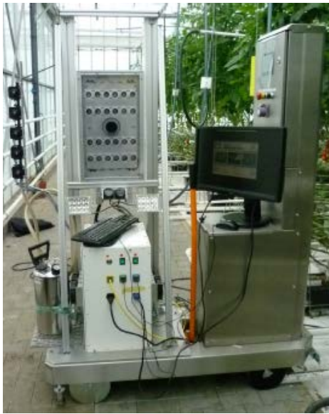
Figure 4.4 Camera system with stereo vision and chlorophyll fluorescence, Side Crop View Platform. Photo courtesy of Gezonde Kas project
