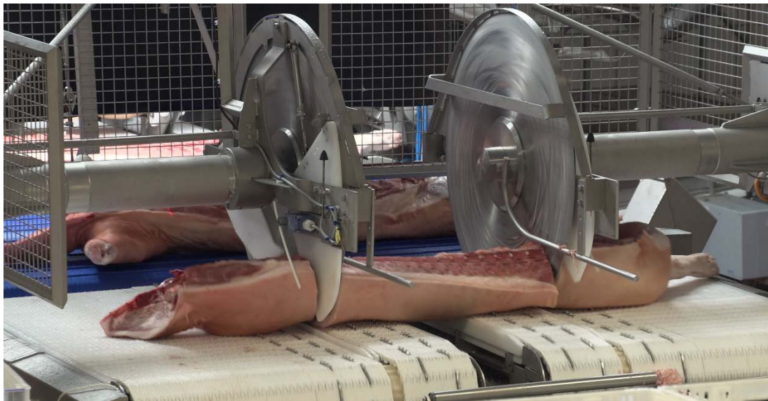
Figure 3.7 Laser-driven cutting positioning for dividing carcasses. Photo courtesy of Marel Red Meat Slaughtering
