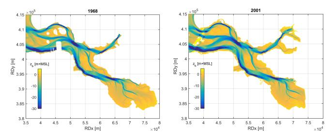
**Figure 10:** Bathymetry of the Eastern Scheldt in 1968 (left), and in 2001 (right). The bed levels are defined with respect to the Amsterdam Ordnance Datum (NAP), which is approximately Mean Sea Level. *Maps by L. de Vet & B. van Prooijen*.
