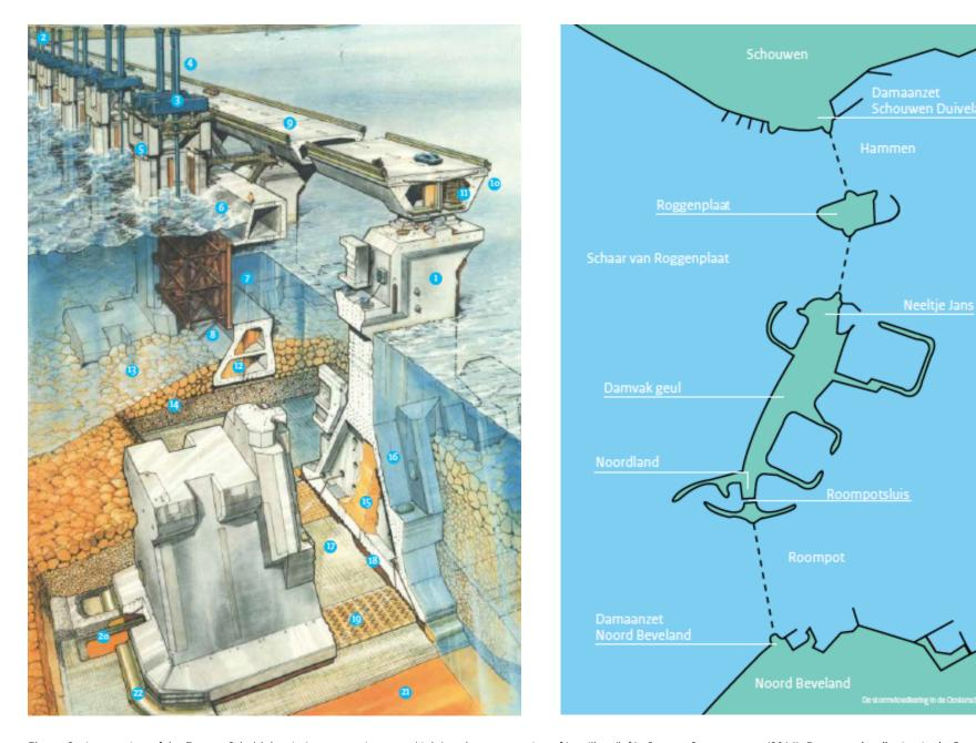
Figure 3: An overview of the Eastern Scheldt barrier's construction parts (right) and a cross section of its pillars (left). Source: Steenepoorte (2014), De stormvloedkering in de Oosterschelde.
