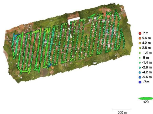
Fig. 3. Camera locations and error estimates. Z error is represented by ellipse color. X,Y errors are represented by ellipse shape. Estimated camera locations are marked with a black dot.
