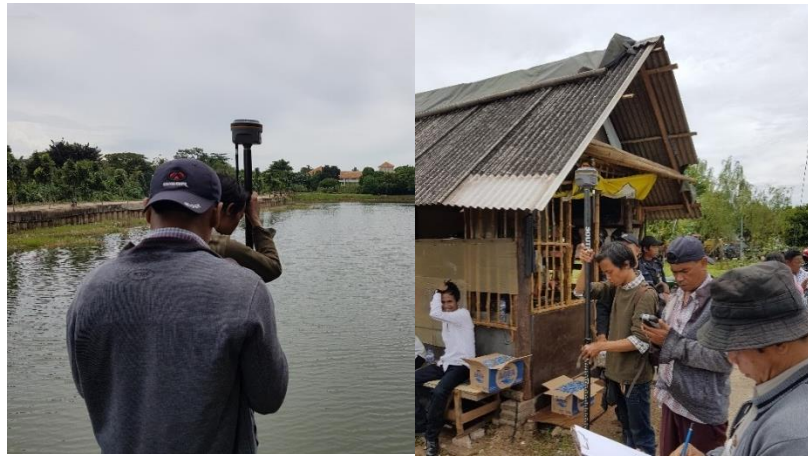
Figure 8. GCPs measuring used GNSS RTK.
