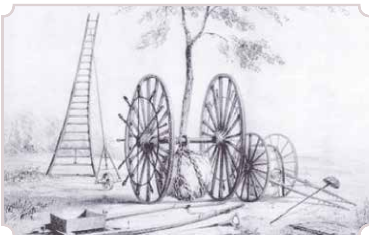
< Foto 2 Mallejan of Treelifter. Bron: The Tree-Lifter , George Greenwood, 1844
