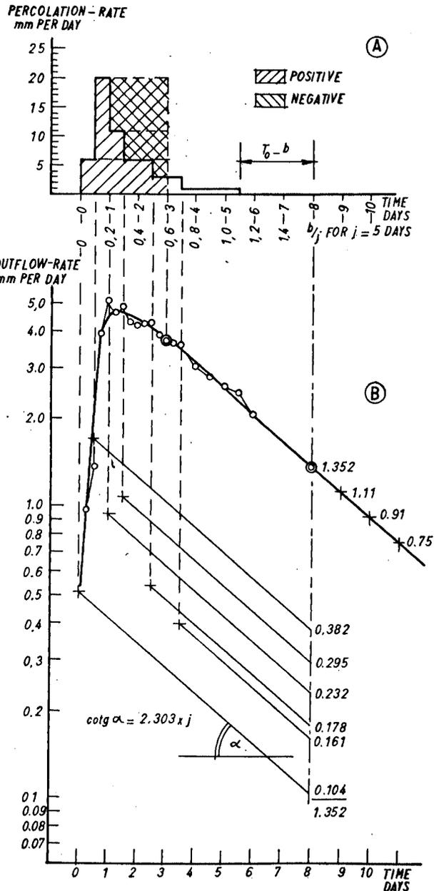
Fig. 4. Computed hydrograph of groundwater-outflow.
