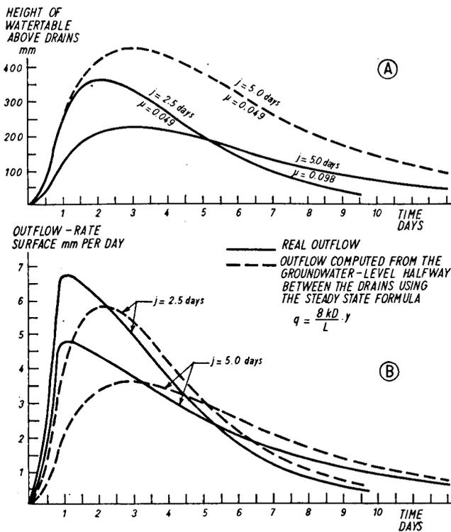
Fig. 5. Error introduced by considering non-steady groundwater-flow as a succession of steady states.
