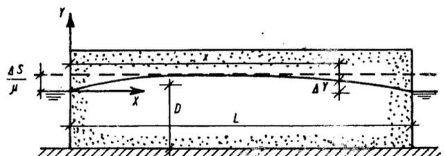
Fig. 1. Two-dimensional flow in a homogeneous soil.
