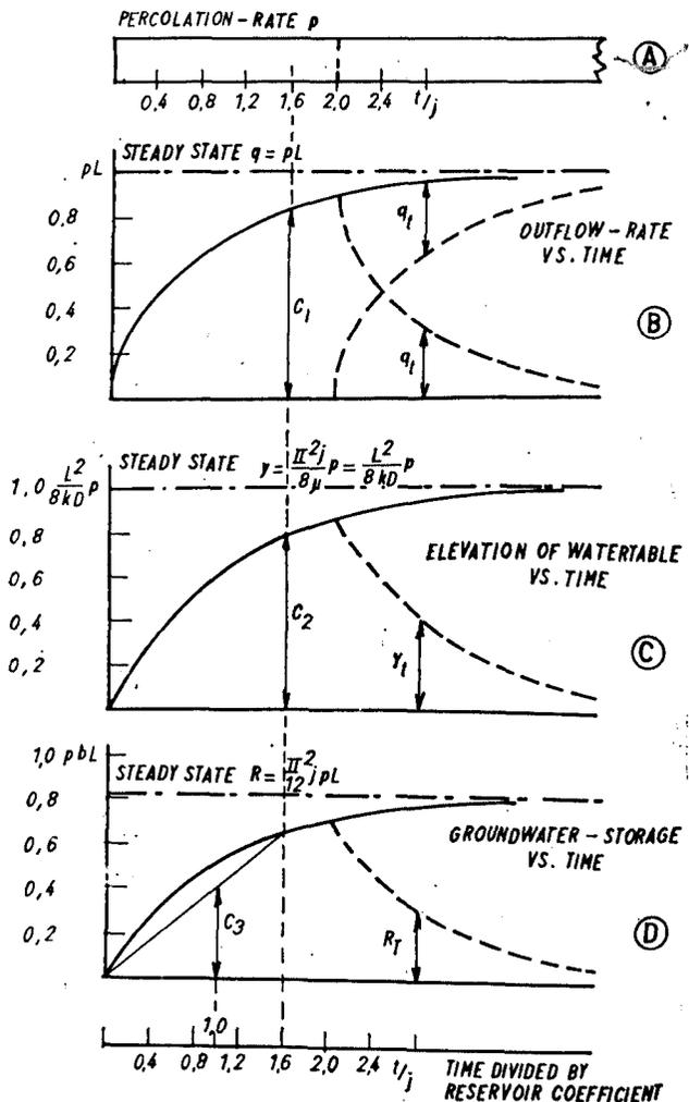
Fig. 2. Groundwater reacting upon steady percolation.
