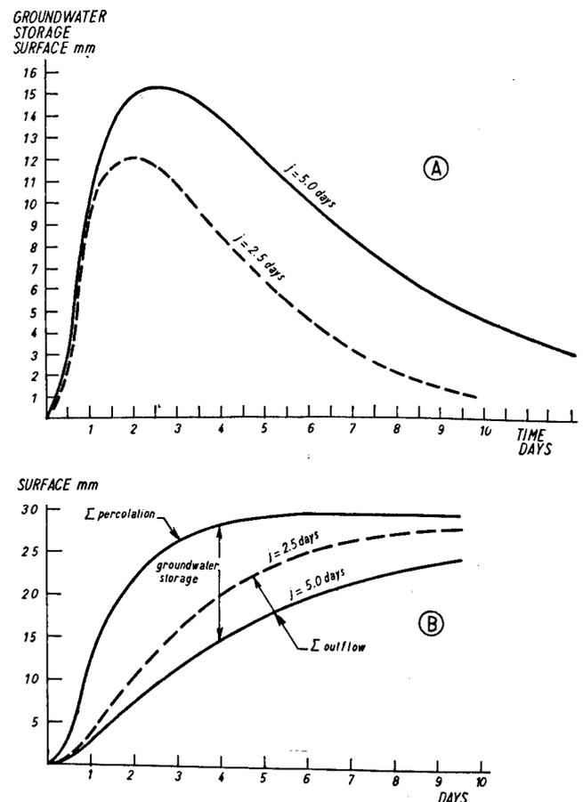
Fig. 6. The reservoir coefficient determines the buffering action of groundwater storage between percolation and outflow.
