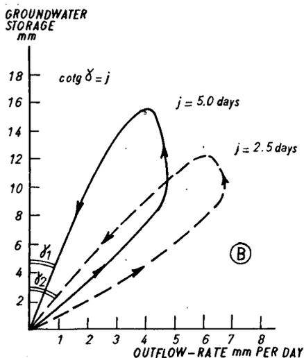
Fig. 7. Only during tail-recession there are fixed relations between the rate of outflow, the height of the watertable and the groundwater storage.
