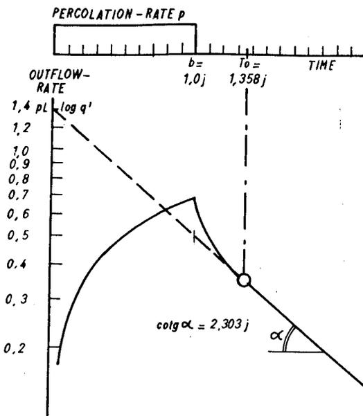
Fig. 3. The depletion curve merges into tail-recession.
