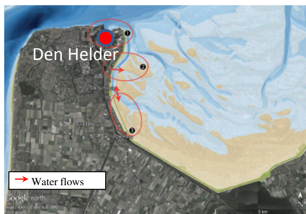
Figure 7. Overview of case study Port of Den Helder with (1) modification of port entrance lay-out, (2) relocation of freshwater discharge and (3) estuarine gradient in Balgzand canal.
