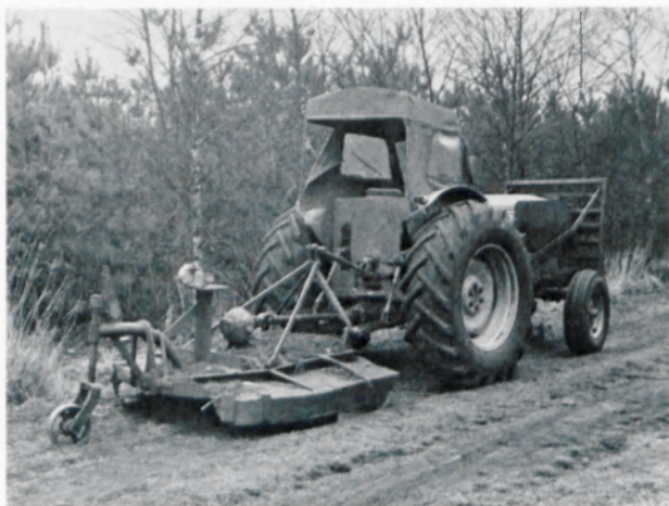
Tending the forest with tractor and rotary cutter (systematic cleaning)
