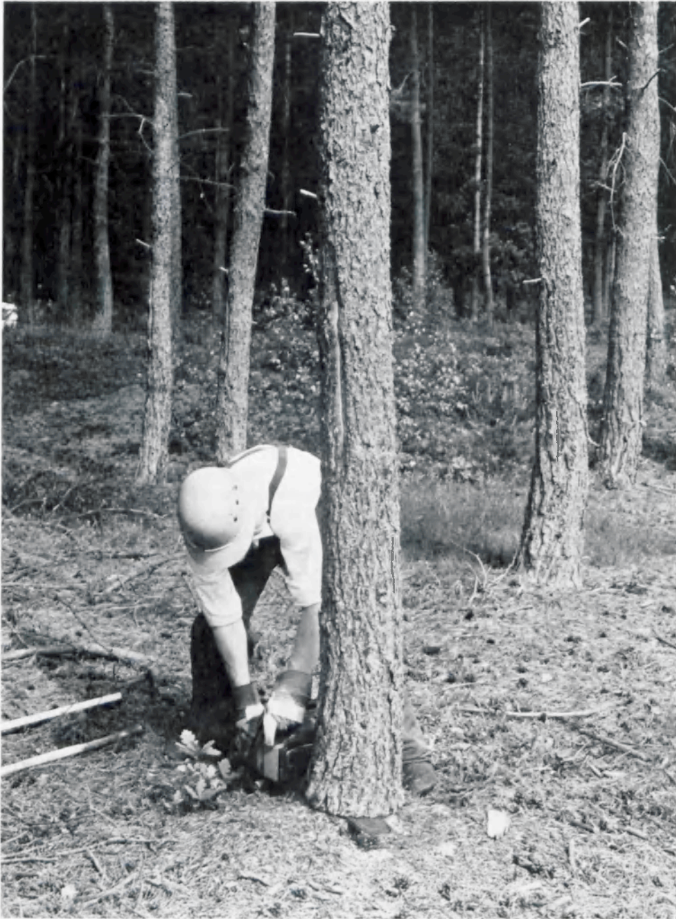
Felling with power saw. Individual means of protection: polyester helmet reinforced with glass fibre, ear caps with neck strap, soft leather working gloves, nylon safety-overall, rubber boots with steel toe-cap, profiled rubber soles and ankle strengtheners.
