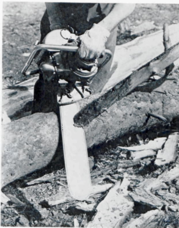
Trimming thick branches with the power saw (thicker than 4 cm at the base)
