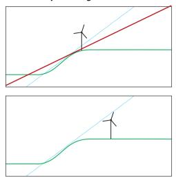
Wind turbines on top of a ridge. Avoid a plateau-edge location to reduce the impression of being overwhelmed when looking up from the valley floor.
