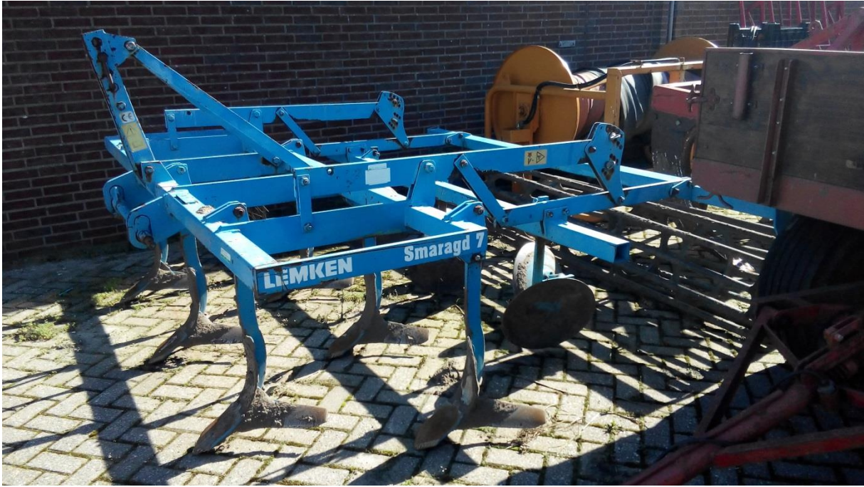
Figure 7 - C: The 'Smaragd', a kind of cultivator, used for non-inversion tillage
