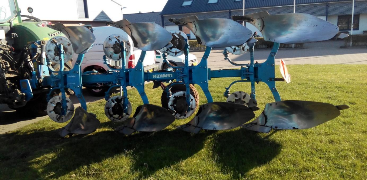
Figure 7 - A: The four-share plough used for conventional tillage
