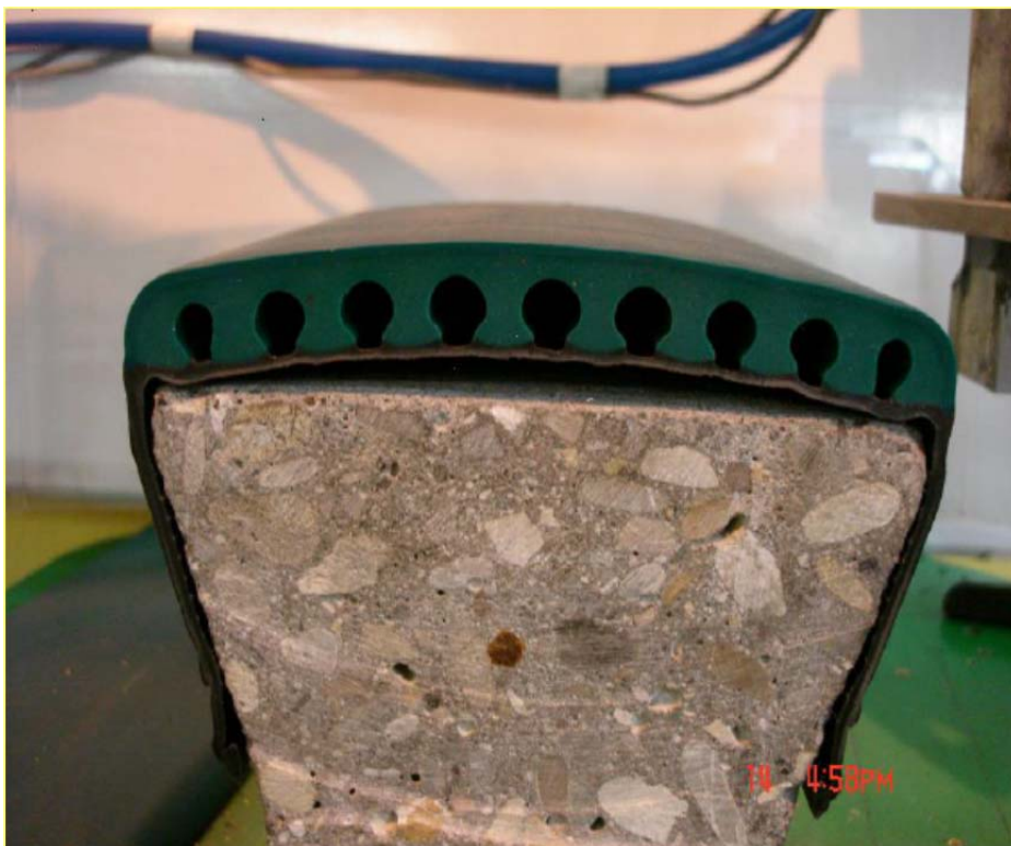
Figure 1 Example of the Comfort Slat Mat on a beam of a concrete slatted floor.
