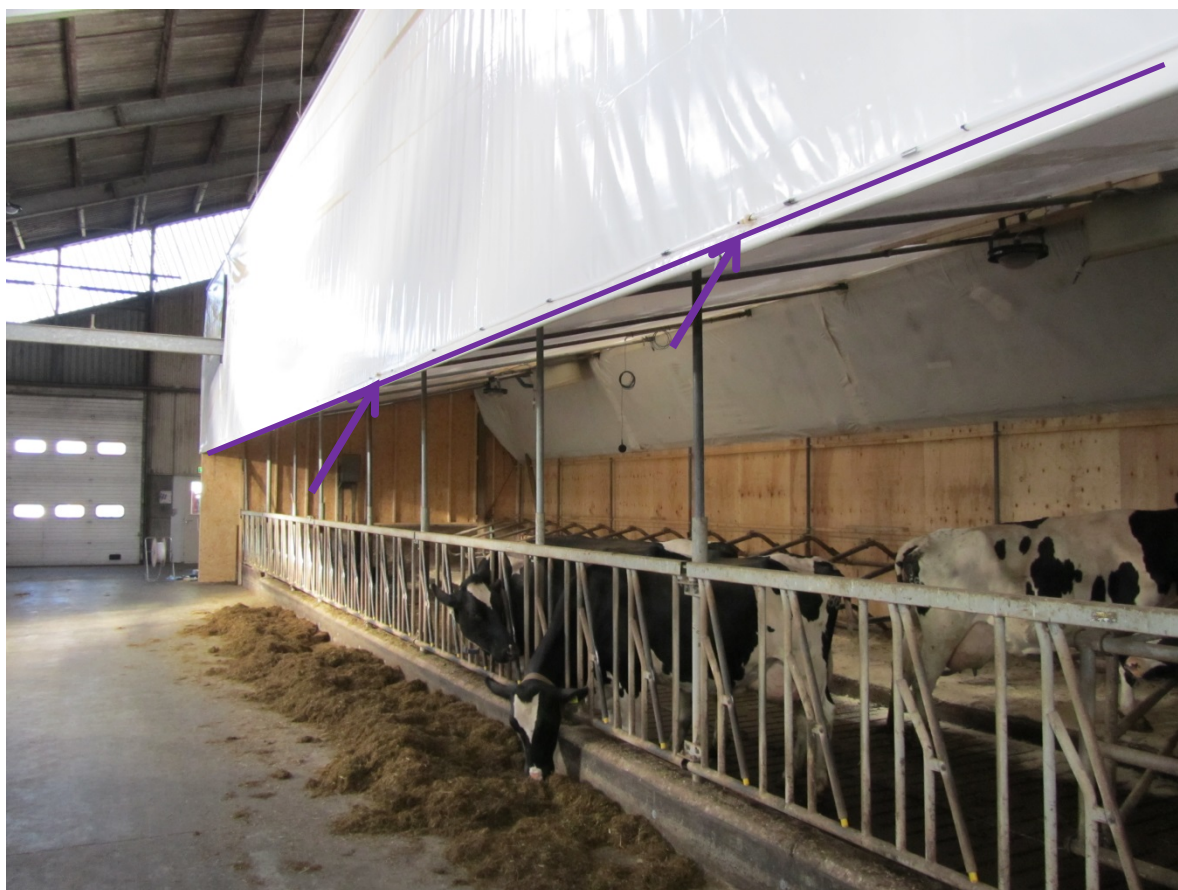
Figure 5 Overview of curtain regulating the incoming air in pulled up position. The purple line and arrows indicates the sampling line with two of the four sampling point along the bottom side of the curtain.
