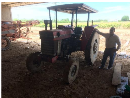
Tractor modified to traditional standards (steel wheels)
