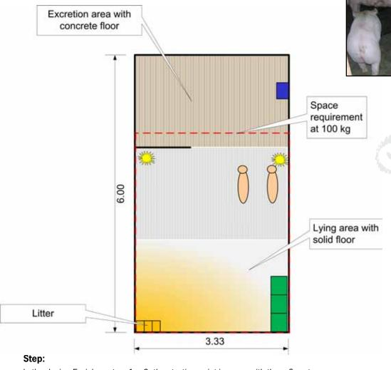
In the design Enrichment on 1 m2, the starting point is a pen with three floor types: a solid floor serving as a resting area, a floor with holes serving as an activity area and resting area for the heavier animals, and a slatted floor serving as a drinking and excretion area. In this case, the floor with holes acts as a multifunctional transitional area. Towards the front of the pen, food and litter are provided; in the middle there are enrichment materials; and water is supplied at the back.
