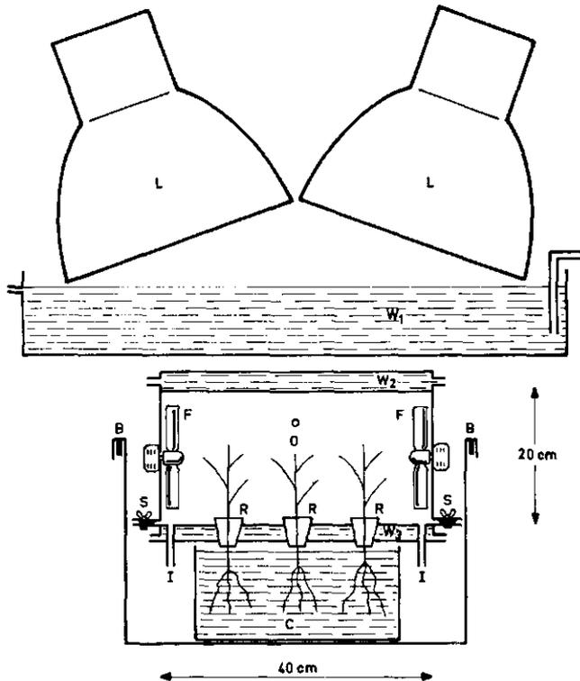
FIG. 1. Diagram of the assimilation chamber and the irradiation of the plants. B = iron bars; C = culture solution; F = fans; I = air inlet; L = lamps; O = air outlet; R = rubber stoppers; S = screws with butterfly nuts; W<sub>1</sub>, W<sub>2</sub>, W<sub>3</sub> = water layers.
