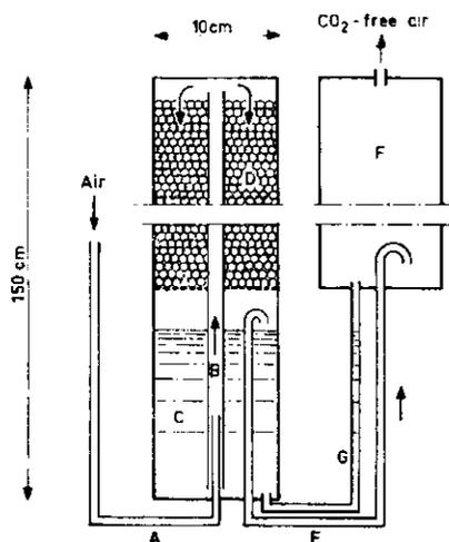
FIG. 2. Diagram of the apparatus for the removal of CO<sub>2</sub> from the air. A = inlet tube for air; B = inner tube; C = potassium hydroxide solution; D = ceramic beads; E = outlet tube for air; F = collecting-vessel; G = tube for flow-back of potassium hydroxide solution to C.
