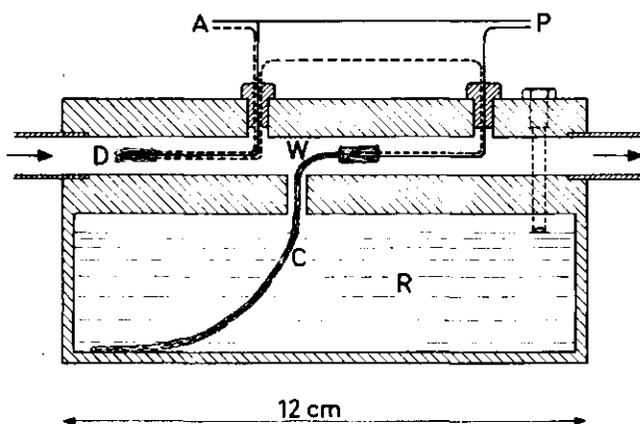
FIG. 5. Diagram of the psychrometer assembly. — = Constantan wires; - - - - = copper wires; D = dry thermocouple; W = wet thermocouple; C = cotton thread; R = reservoir with distilled water. The air stream is in the direction of the arrows. The air temperature is measured between the wires at A, and the psychrometer value between the wires at P.
