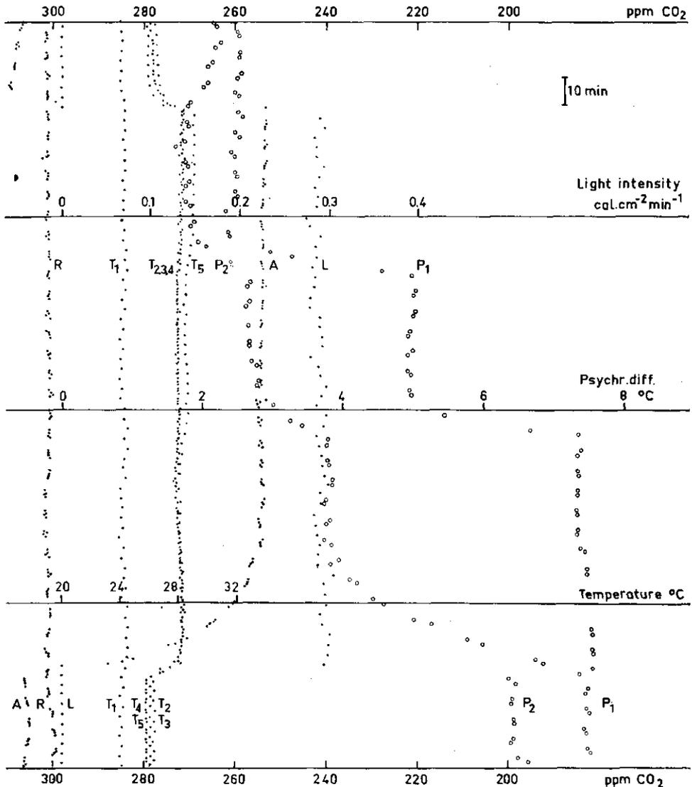
FIG. 9. Recorder chart ( $\frac{6}{10}$  actual size) of an experiment with beans at different humidities. The scales for CO<sub>2</sub> concentration, light intensity, psychrometer value, and temperature are indicated in the figure. The symbols in the different records are the same as those in Fig. 7 (P<sub>1</sub> and P<sub>2</sub> being the psychrometer values of the air at the inlet and outlet sides of the assimilation chamber, respectively).
