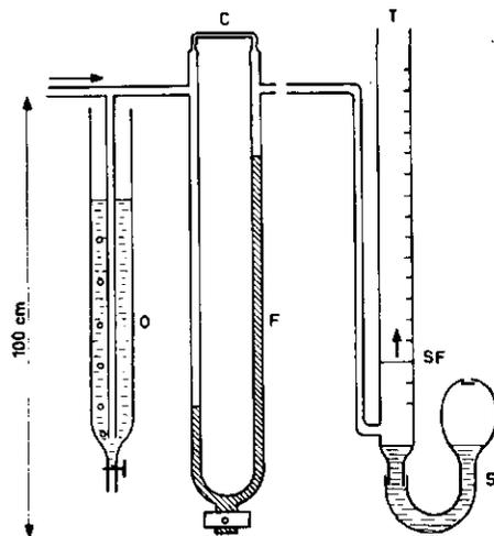
FIG. 3. Diagram of the arrangement with a flow meter. C = capillary tube; F = flow meter with coloured liquid; O = overflow. On the right side the calibration device for low flow rates. S = soap solution; SF = soap film; T = burette.
