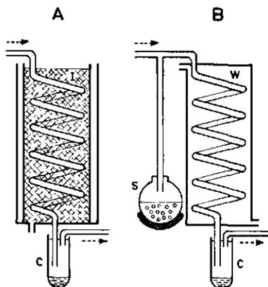
FIG. 4A. Drying condenser. I = ice; C = vessel for condensed water. The air stream is in the direction of the arrows. FIG. 4B. Humidifier. S = steam vessel; W = water; C = vessel for condensed water. The air stream is in the direction of the arrows.
