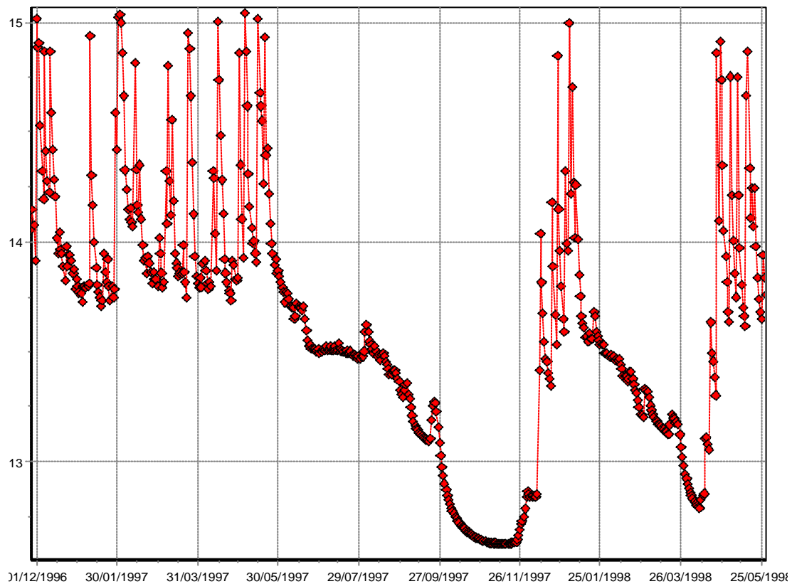
Figure 4.19. X-axis: calculated water levels in the Sungai Sebangau off Plot1B ( m +msl) in 1997. Y-axis: days
