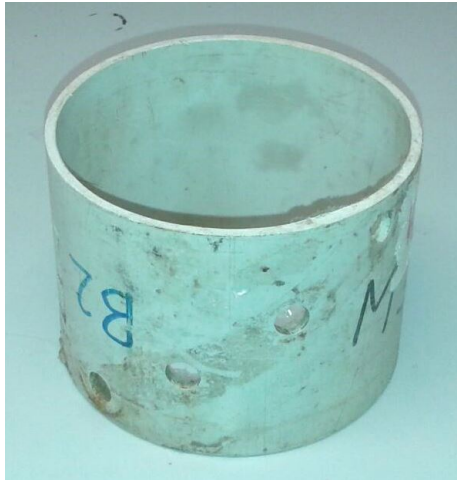
Figure 4.3: The PVC rings in which the soil samples were kept for the evaporation method.
