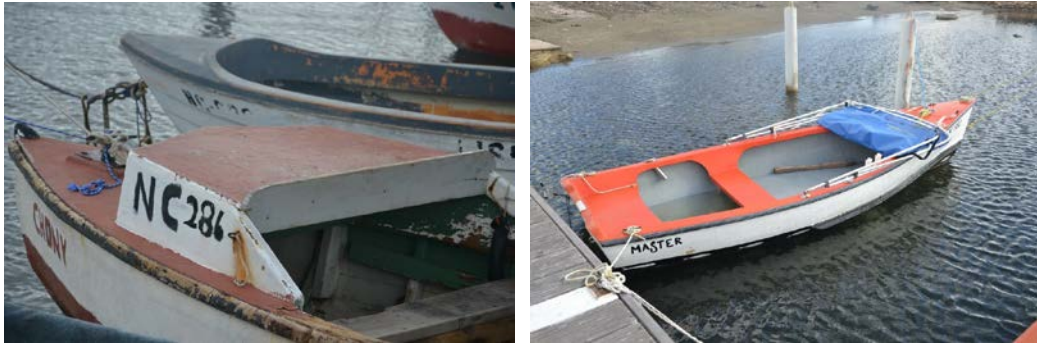
Figure 3.2: Two smaller vessels with 'a guard', protecting the fishers at sea against the waves.
