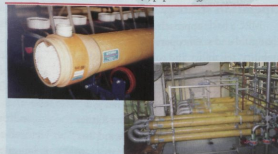
Fig. 2: COMPACT membrane bioreactor application: (a) membrane module, (b) paper mill effluent.
