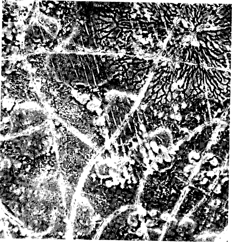
Fig. 4. Cellophane recovered from forest soil (mor) attacked by fungi (fanlike growth and hyphae), Cytophaga , and slugs or snails. 390 \times .
