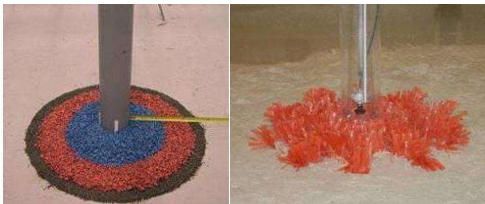
Figure 7.9 (Left) An example of a scale model test for scour protection consisting of loose rock: a top layer of red and blue rock (armor layer) and a bottom layer of black rock (filter layer); (right) an example of a scale model test for scour protection consisting of frond mats (artificial seaweed)
