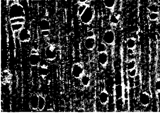
Engelhardtia serrata transverse surface (×20)
