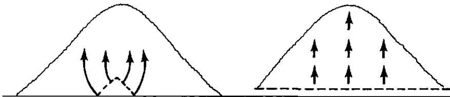
Fig. 71. Potato piles with provisions for improving convective ventilation.
