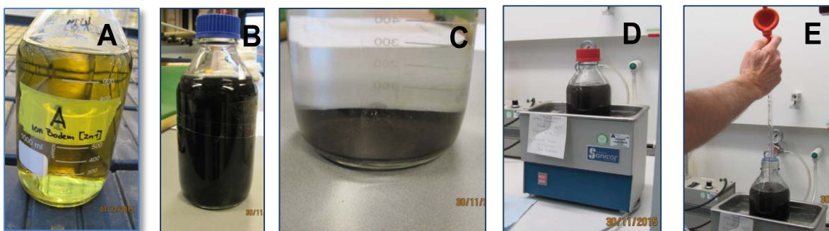
Figure 6-1. Aqueous solutions of micronutrients. A. In ionic form, B. suspension of micnobits just after shaking, C. suspension of micnobits after precipitation, D. suspension of micnobits during ultra-sonication and E. taking samples from micnobit suspension just after sonication
