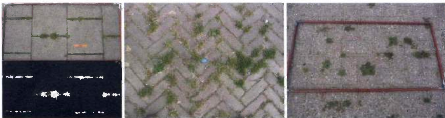
Fig. 1. Images of pavements on which herbicide use was tested: concrete tiles (left top), red brick (middle) and grey brick (right). Also a green pixel image (4% green) of top left picture is shown.
