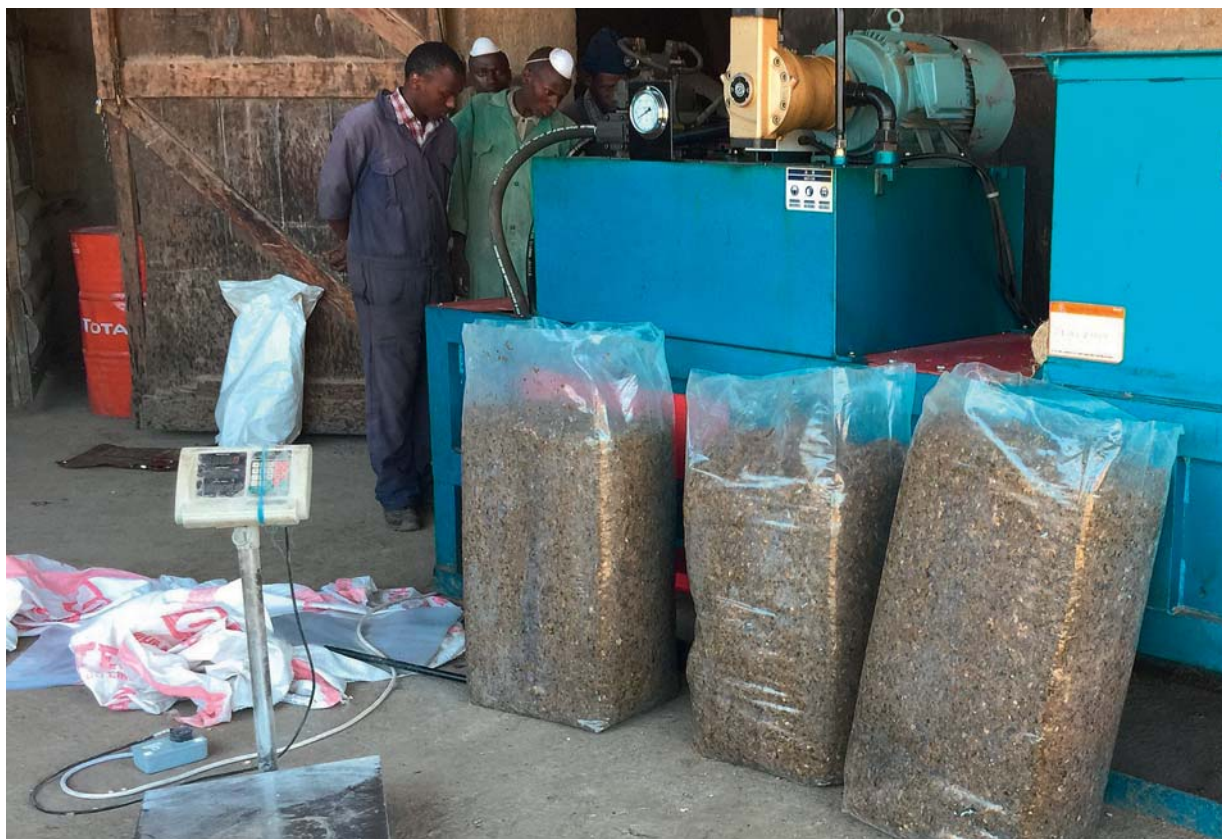
The packaging machine that produces maize silage briquettes.
