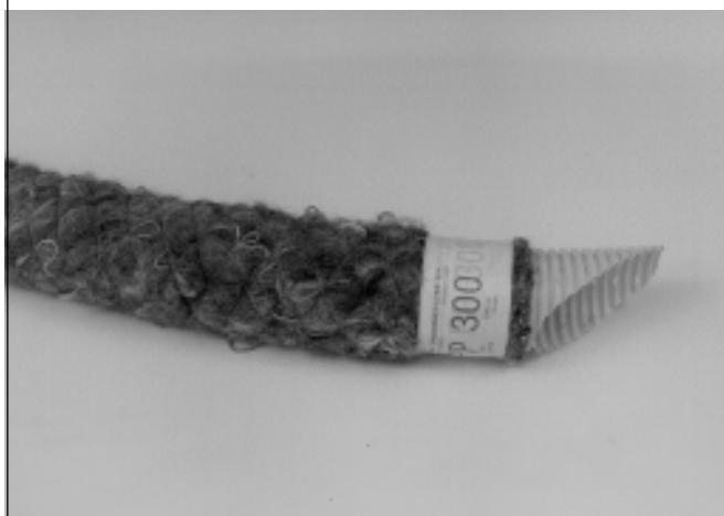
FIGURE 17 PLM envelope made from polypropylene waste fibres (PP-300)
