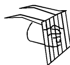
Permanently fixed vermin grating
