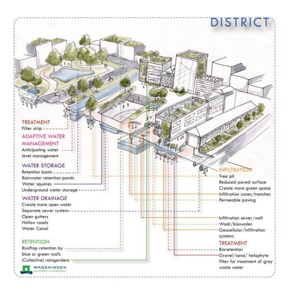
Figure 3.3 Illustration of possible Water Smart measures on district scale
