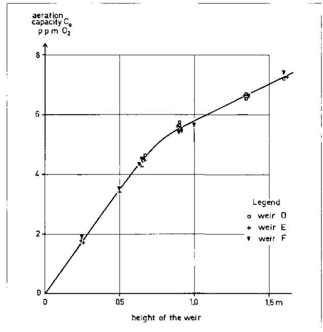
Fig. 14 - Effect of height on the aeration capacity at weirs D, E and F measured at a flow rate of  $40 \text{ m}^3 \cdot \text{hr}^{-1} \cdot \text{m}^{-1}$  and 0.6 m depth of receiving basin.
