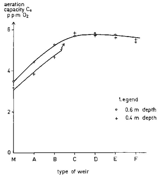
Fig. 16 - Effect of depth of the receiving basin on the aeration capacity at different weirs measured at a weir height of 0.90 m and at a flow rate of  $40 \text{ m}^3 \cdot \text{hr}^{-1} \cdot \text{m}^{-1}$ .
