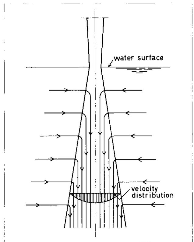
Fig. 4 - Spreading of the submerged jet over the depth of the receiving basin. (After Häusler - 1961).
