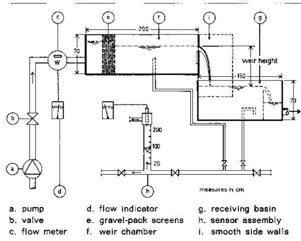
Fig. 7 - Experimental installation.
