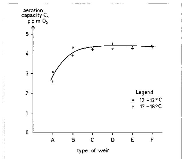
Fig. 9 - Effect of temperature on the aeration capacity at different types of weirs measured at a weir height of 0.65 m, a flow rate of 40 m<sup>3</sup>.hr<sup>-1</sup>.m<sup>-1</sup> and at 0.6 m depth of receiving basin.
