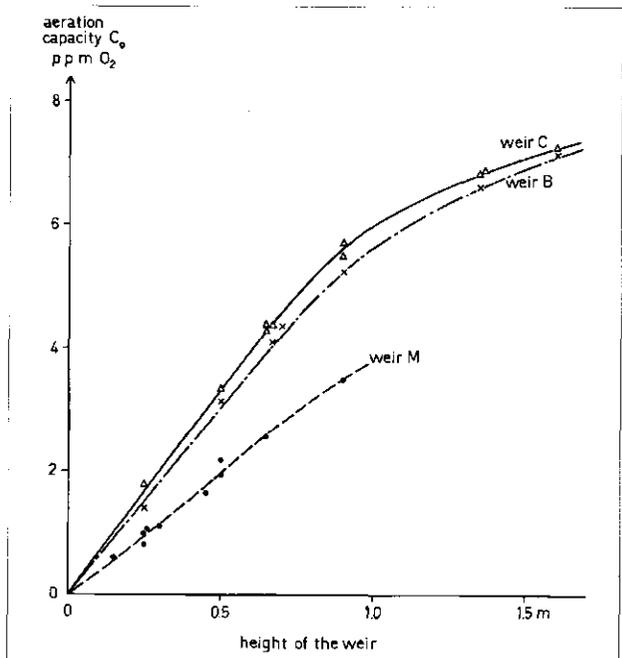
Fig. 12 - Effect of height on the aeration capacity at weirs M, B and C measured at a flow rate of  $40 \text{ m}^3 \cdot \text{hr}^{-1} \cdot \text{m}^{-1}$  and 0.6 m depth of receiving basin.
