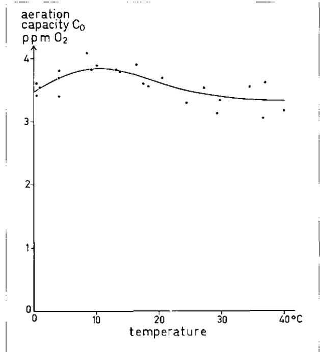
Fig. 2 - Effect of temperature on the aeration capacity (after Gameson, A. L. H., Vandyke, K. G. and Ogden, C. G. - 1958).
