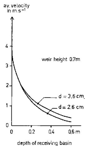
Fig. 6a - Relationship between av. downward velocity of submerged jet and depth of receiving basin for jets at 2.6 cm diameter (after Häusler).
