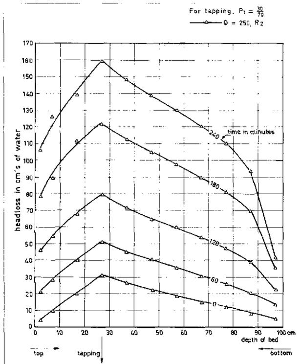
Fig. 3 - Head loss VS depth of bed.
