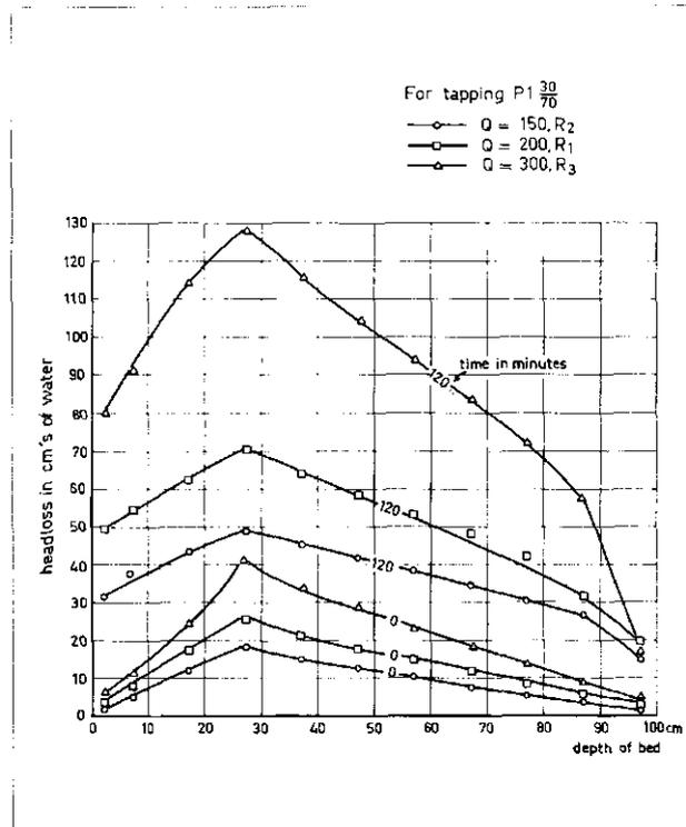
Fig. 4 - Head loss VS depth of bed.
