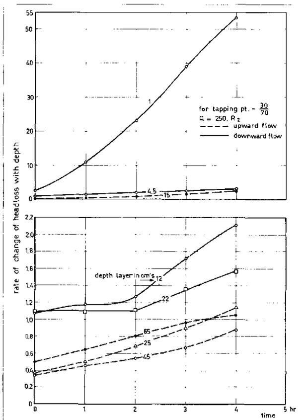
Fig. 5 - Rate of change of headloss with depth VS time.
