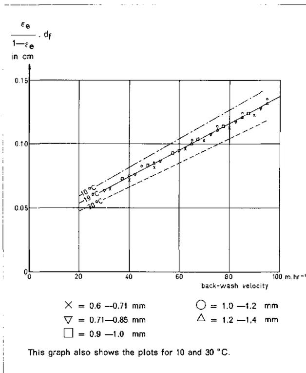
Fig. 9 - Relative sand-bed expansion as a function of backwash velocity for grain sizes varying from 0.6 to 1.4 mm. For these sizes a single relationship has been adopted as is shown for data obtained at sand-beds with heights of 50 to 80 cm at 19 °C.
