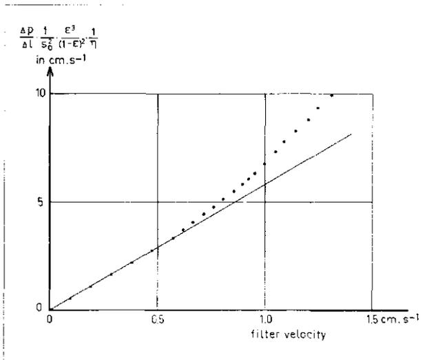
Fig. 4 - Resistance to flow of stainless steel balls ( $d = 2.5 \text{ mm} \pm 0.01$ ). Height of the bed was 49.7 cm and porosity was 41.5 per cent.
