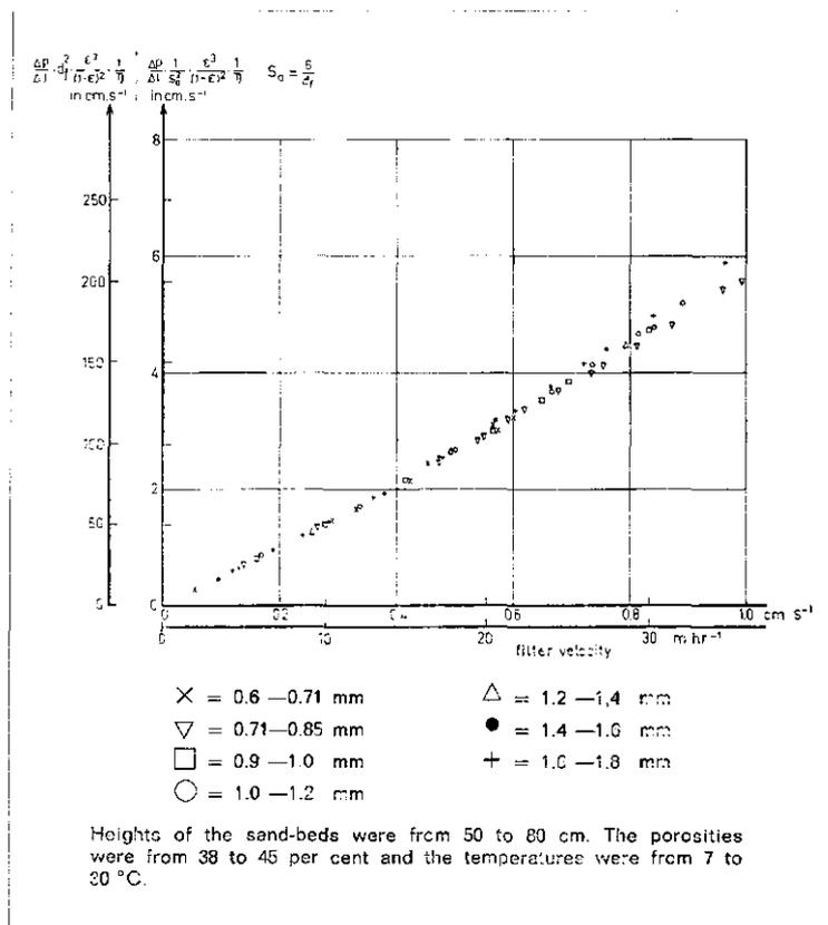
Fig. 8 - Resistance to flow of homogeneous sand samples.
