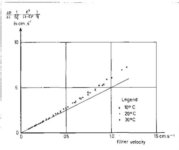
Fig. 7 - Modified resistance coefficients for homogeneous sand ( $d_s = 1.095 \text{ mm}$ ) at different temperatures.
