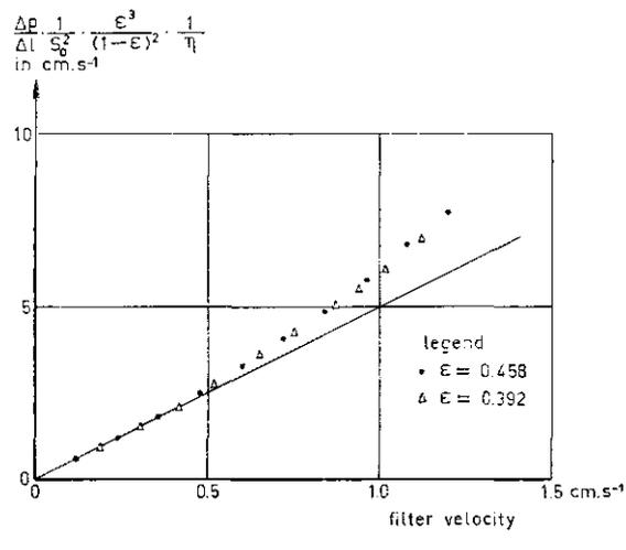
Fig. 5 - Resistance to flow of homogeneous sand ( $d_s = 1.69 \text{ mm}$ ) at different porosities.
