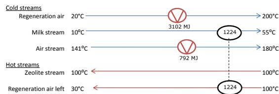
Fig. 4. Heat exchanger network of scenario 3, with the corresponding temperatures and amounts of heat exchanged.
