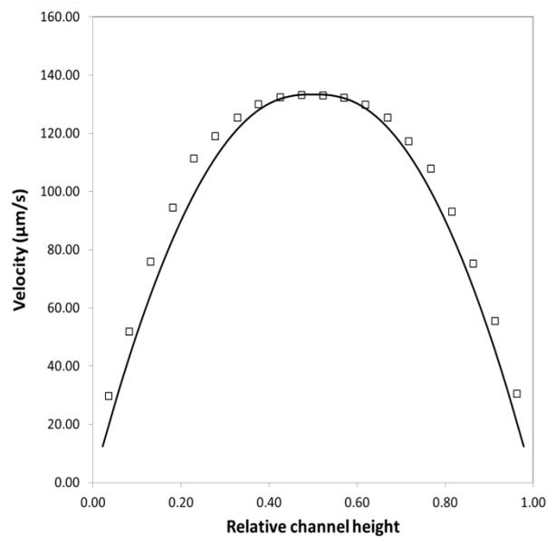
**Figure 3. Velocity vs. the relative channel height, for  $\phi_{bulk} = 0.3$ . Experimental results by T.X. van de Laar ( $\square$ ); Our model results (line).**
