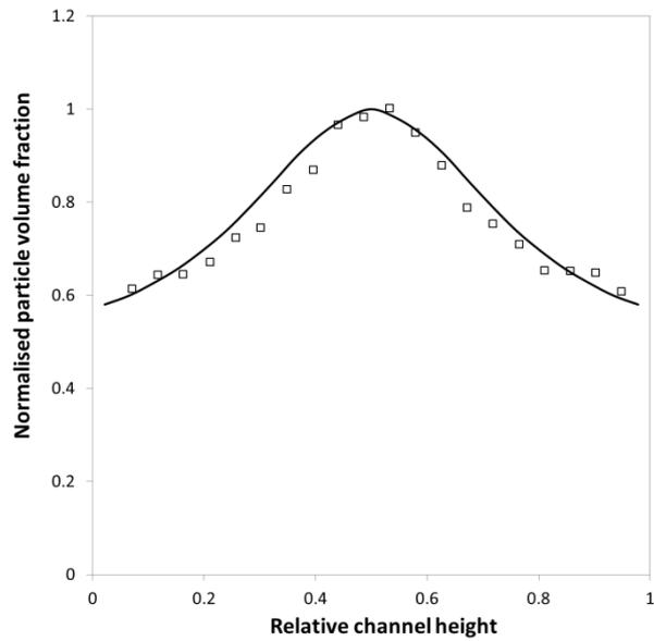
**Figure 2. Normalised particle volume fraction (relative to the highest value) vs. the relative channel height, for  $\phi_{bulk} = 0.5$ . Experimental results by T.X. van de Laar ( $\square$ ); Our model results (line)**
