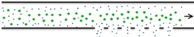
**Figure 1. Schematic view on fractionation due to shear induced diffusion**
