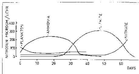
Fig. 2 - The decomposition of nitrogenous organic matter in mixed plankton, showing the appearance of soluble nitrogen compounds in the water in which it is suspended (See v. Brand).
