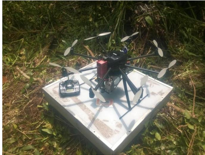
Figure 3. The UAV mounted with the HYMSY
