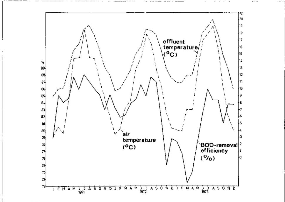
Fig. 11 - The influence of wastewater temperature on the BOD-removal efficiency at the Utrecht trickling filter plant [8].
