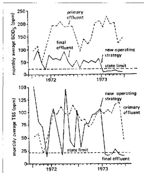
Fig. 13 - The influence of a new operating strategy on the effluent quality at the Hillsboro contact stabilization plant [9].
