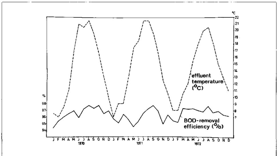
Fig. 12 - The influence of wastewater temperature on the BOD-removal efficiency at the Amsterdam activated sludge plant [8].
