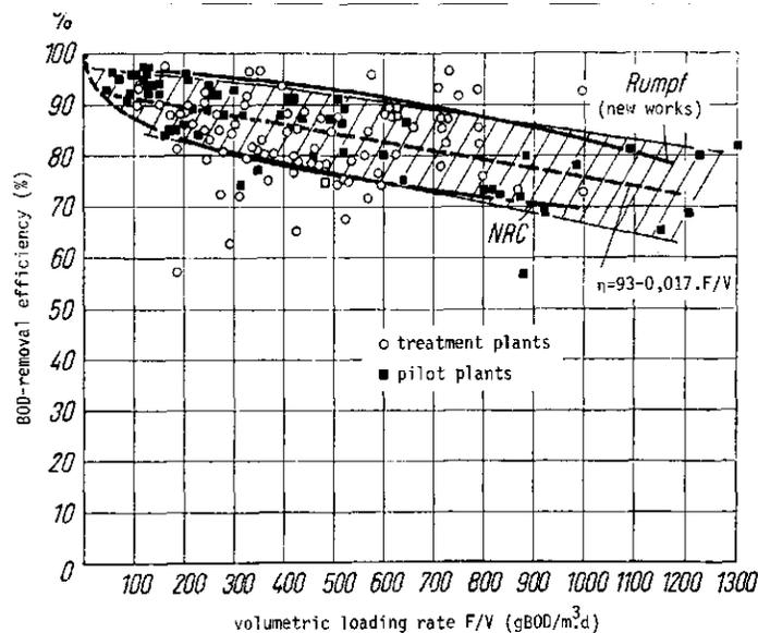
Fig. 2 - The influence of the volumetric loading rate on the BOD-removal efficiency [11].
