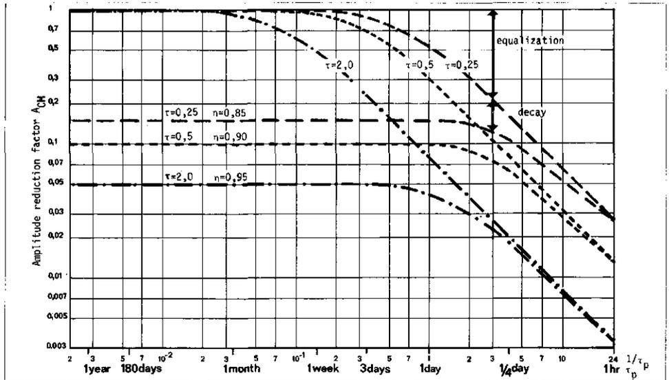
Fig. 7 - The influence of retention time  $\tau$  and treatment efficiency  $\eta$  on the amplitude reduction factor  $A_{CM}$  at various input periods  $\tau_p$ .
