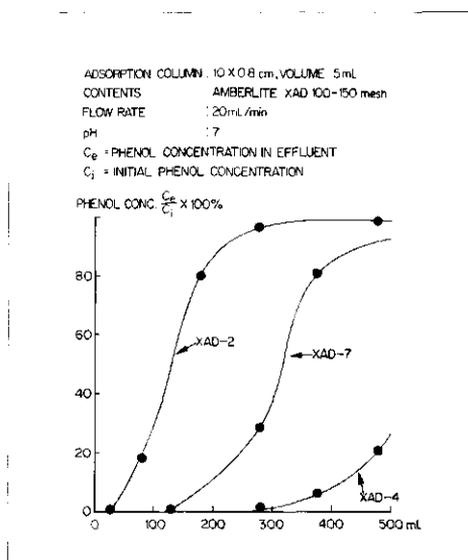
Fig. 2 - Adsorption of phenol on amberlite resins: break-through curves for 10 mg/l solutions.
