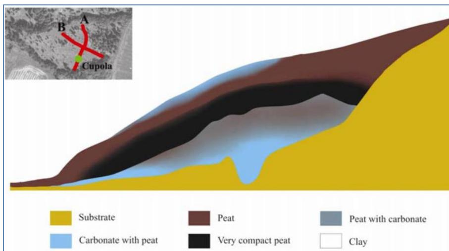
**Figure A2.6: Relief of the soil surface and the thickness of the peat en travertine deposits** (Maderas et al. 2012).
