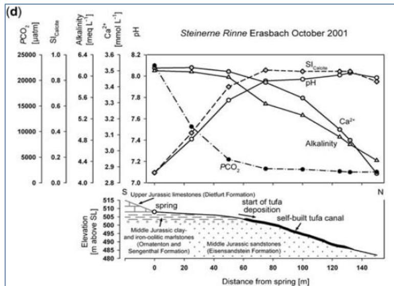
**Figure 2.4: An example of the downstream changes in CO<sub>2</sub> pressure (pCO<sub>2</sub>) calcite saturation (SI<sub>calcite</sub>) Alkalinity, Calcium concentration and pH along a stream with travertine deposition (after Arp et al. 2010)**
