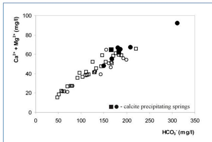
**Figure 2.3: Summary of Ca, Mg and  $\text{HCO}_3^-$  content of water from springs (Smieja & Smieja-Król 2007) which shows that petrifying springs in Poland have usually Ca + Mg content higher than 50 mg/l and  $\text{HCO}_3^-$  contents higher than 150 mg/l.**
