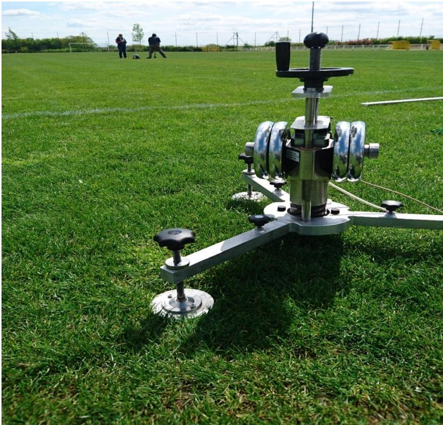
The torque (EN 15301-1:2007) simulates the grip provided by the surface during a player's change of direction
