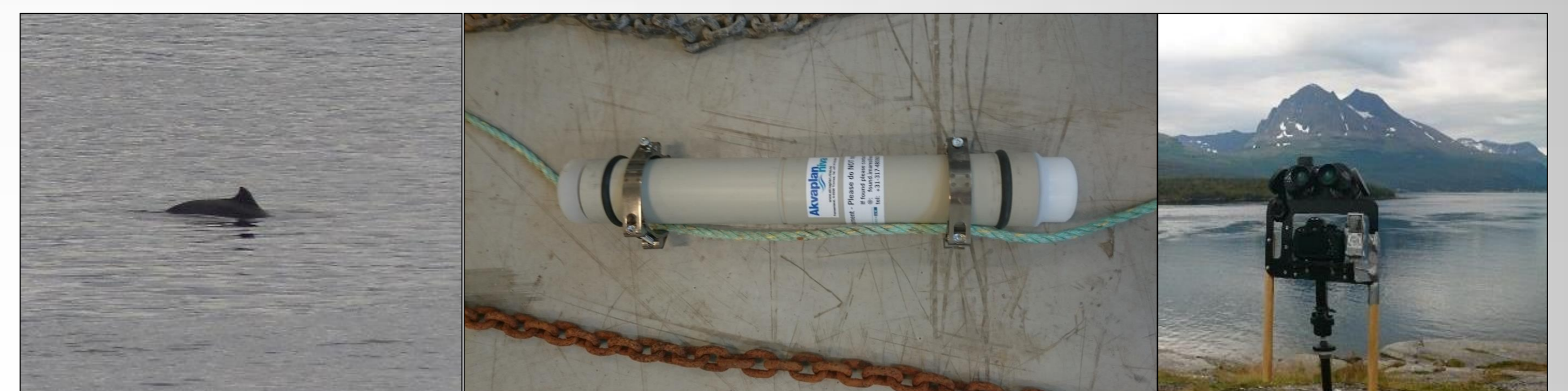
Fig. 2 From left to right: a harbour porpoise in Rystraumen, a C-POD and the camera system used to track harbour porpoises from the observation point. Photos: R. Smit
